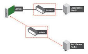
The minimum AccuSense Control system consists of an AccuSense Control, one AccuSense Radio, and a isolator. The system can also consist of two AccuSense Radios with an isolator for each AccuSense Radio that offers electrical isolation up to 1500V, surge protection up to 1500V, and AC power cross protection.
