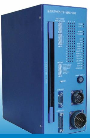
▷ The Model MMU-1600 is a full-featured unit that monitors up to 16 traffic signal channels for conflicting inputs, improper sequencing, incorrect timing, and invalid signal voltage levels.
